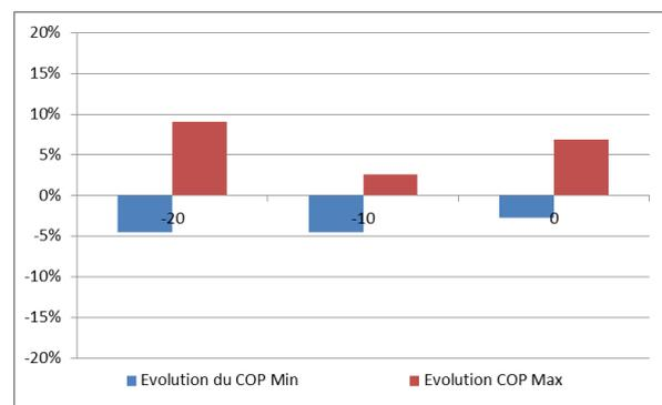
Figure 13-9: Evolution of COPs of units when replacing R-404A by R-452A.
