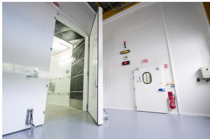
Figure 13-7: Climatic tunnel for testing of refrigeration units for refrigerated transport.
