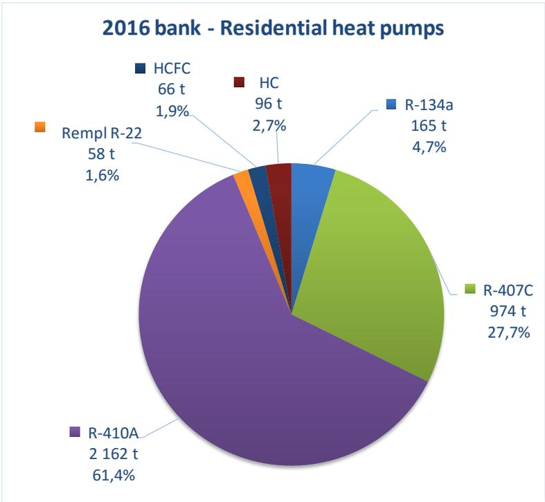
Figure 8-1: Sharing of refrigerants used in HPs and represented in the 2016 bank (air / water, water / water, ground / water & ground / ground).
