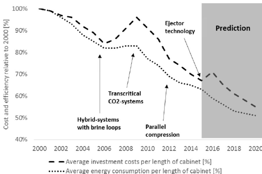
Figure 6-4 – Evolution of costs and energy consumptions of CO<sub>2</sub> systems in commercial refrigeration. Feedback from Switzerland (European Commission, 2017).
