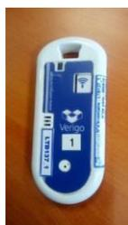
Figure 13-2 : Temperature and humidity recorder.
