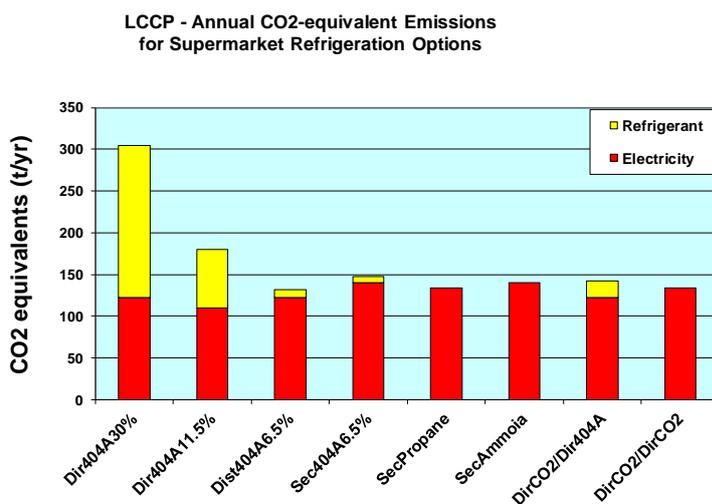
Figure 6-3 – Comparison of the total annual equivalent CO<sub>2</sub> emissions of several types of commercial refrigeration plants (*Bivens, 2002*).
