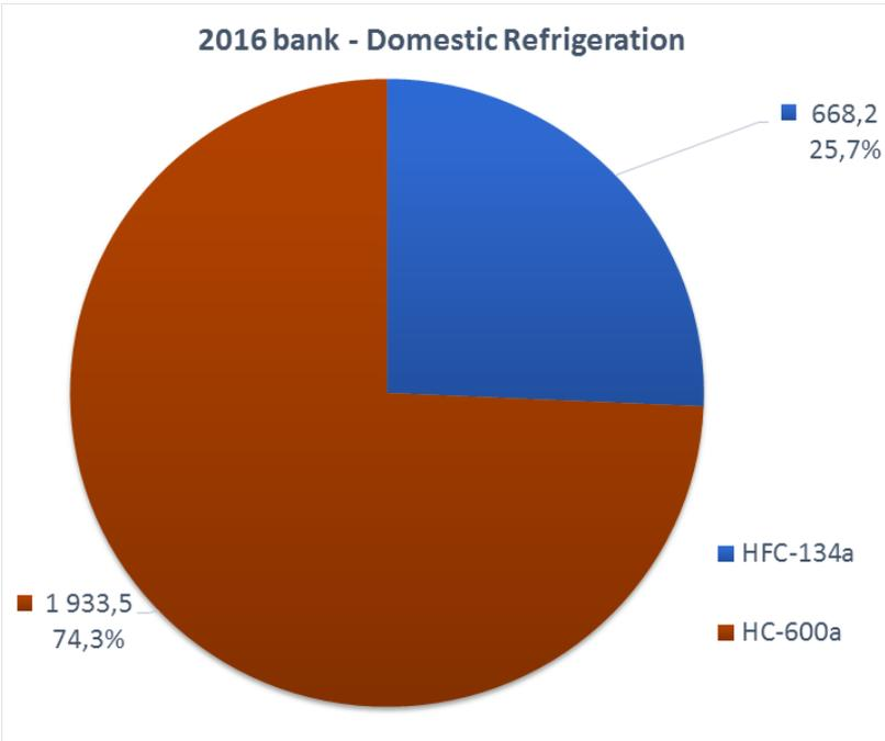
Figure 5-1: Shares of refrigerants used in the domestic refrigeration bank in 2016. (Barrault 2016)
