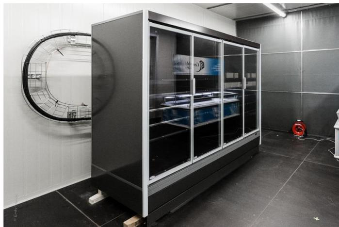
Figure 13-11: Climatic test room for refrigerated display case.
