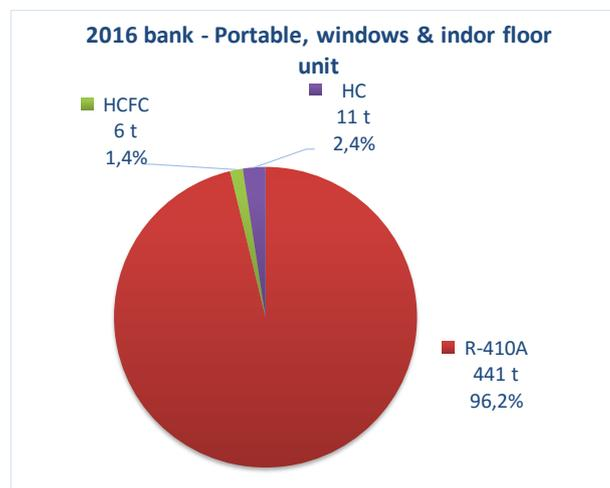
Figure 7-1: Bank 2016 – Hermetic air-conditioning systems.
