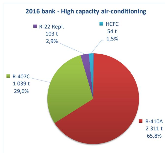
Figure 7-3: Bank 2016 –Multi-splits systems, DRVs and rooftops.
