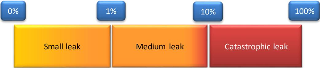
Figure 3-5: Leak typology as a function of leak diameter/piping diameter ratios.
