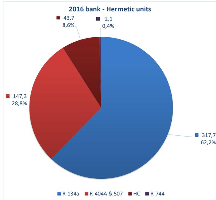
Figure 6-1 – Hermetically sealed equipment (small stores) – 2016 bank.
