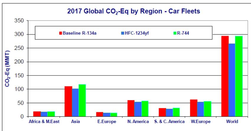
Figure 9-1: Evaluation of total equivalent CO<sub>2</sub> emissions (direct + indirect LCCP meaning) of fleets of mobile air conditioners assuming the implementation of alternatives to all new vehicles as of 2011 (Source: Papisavva, 2014).
