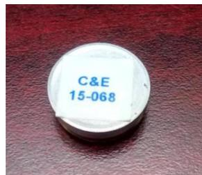
Figure 13-1: Temperature recorder.
