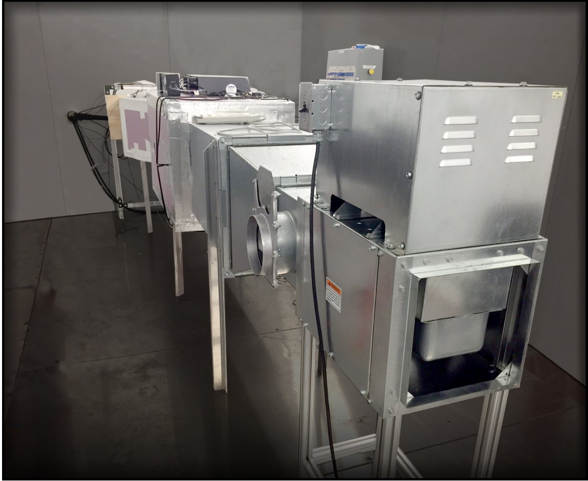
Figure C.4. R-22 indoor air enthalpy tunnel fully instrumented and connected to the data acquisition system.
